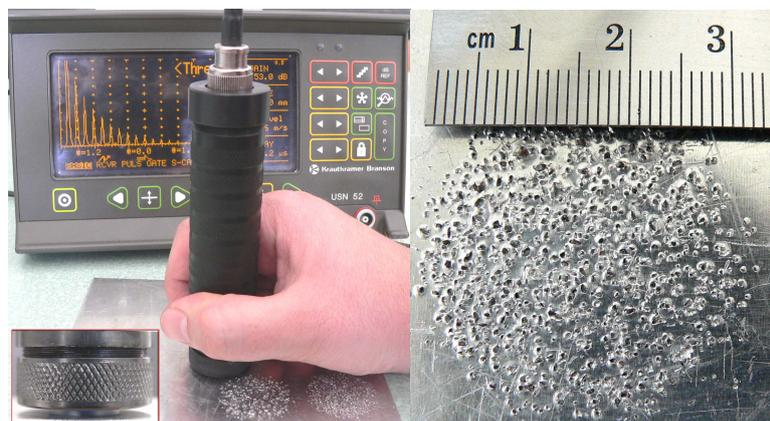
Fig.15. Practical application of a proposed device and aluminium rough-plate
